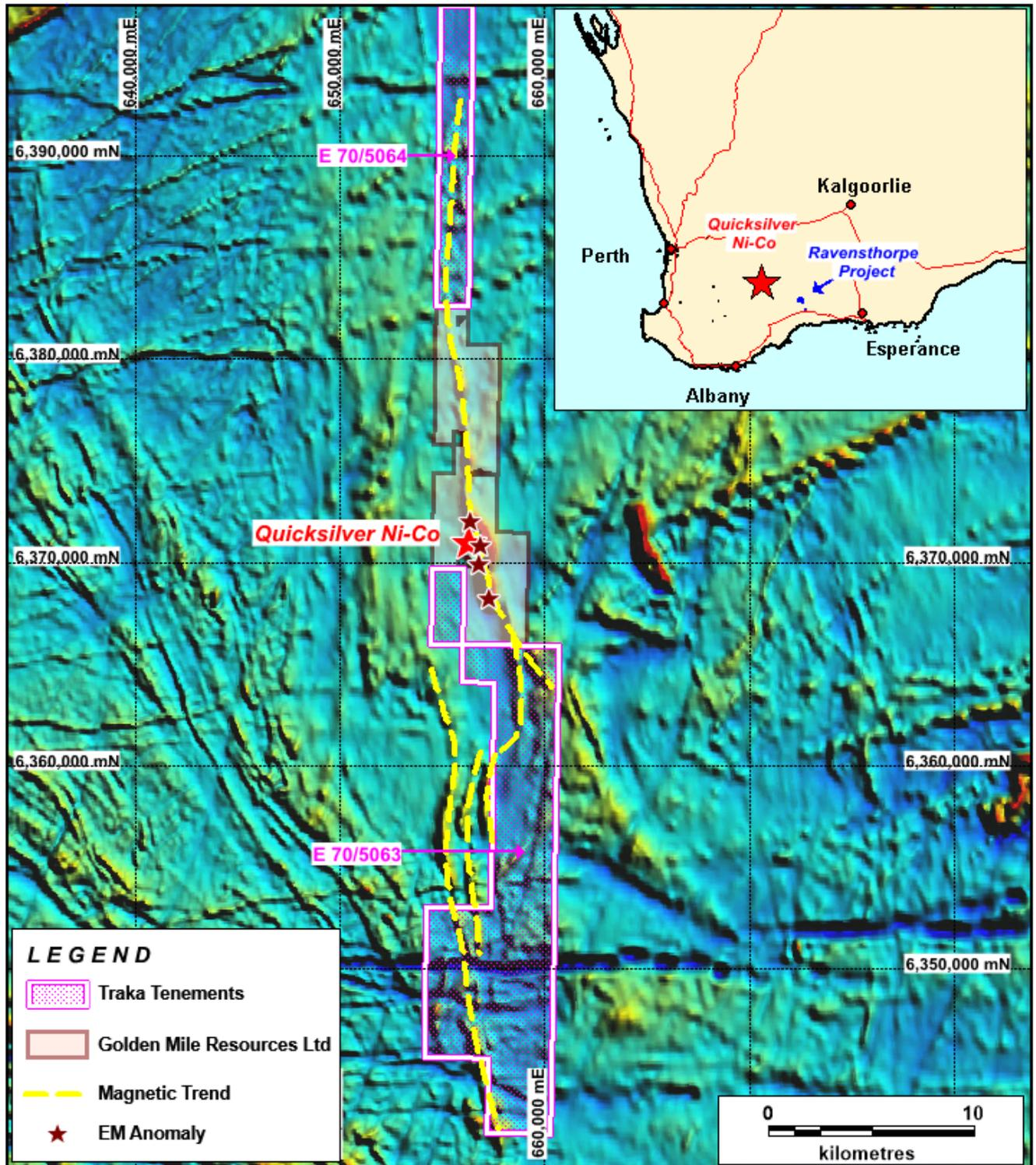
Figure 1. An aeromagnetic image showing Traka's tenements north and south of the Quicksilver project and the location of Golden Mile's four EM targets.
